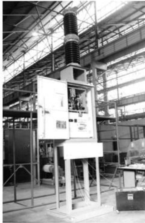
Fig. 3.14: 25 kV outdoor track-side vacuum switchgear
